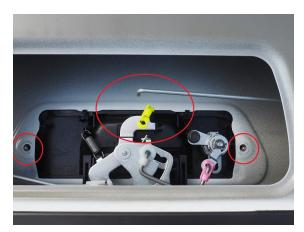
4) Disconnect the Rod from the back of the key barrel and remove the pink plastic clip
