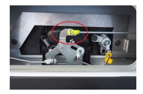
7) Attach the wiring loom to motor. Black to Blue—Red to Red
