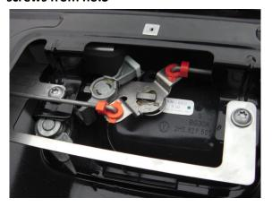
4) Connect wiring loom to the actuator:
