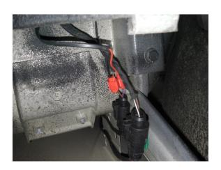
5) Feed Cables out of tailgate and strap tight using cable ties, Feed out towards the side the fuel filler cap is.
