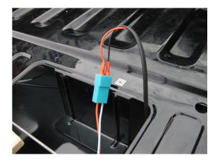
7) Feed cable through bumper, either drill a small hole or you can squeeze the cable through a gap on the left side of the bumper. Use the plastic Sheaving to protect the wire
