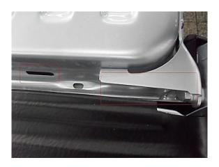
8) Connect the wiring loom to the vehicles central locking, This is found on the under side between the wheel arch and back of truck
