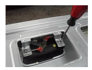
3) Install the base plate and actuator kit, hold in place by replacing the removed screws from no.3
